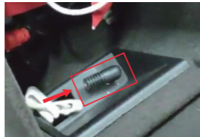
27. 注意需要将CarPlay的AUX插头连接到原车的AUX端口上 Note that the AUX plug of CarPlay needs to be connected to the AUX interface of the original car
