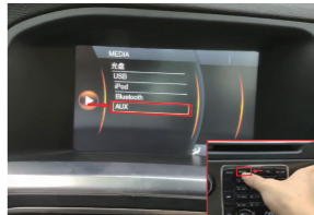
29. 通过原车MEDIA键进入媒体界面，选择AUX Enter the media interface of the original car system through the MEDIA button, select AUX
