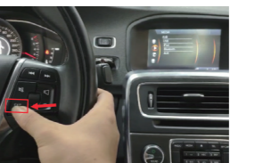
3. 长按方向盘上的EXIT键切换CarPlay系统 Long press the EXIT button on the steering wheel to switch the CarPlay system
