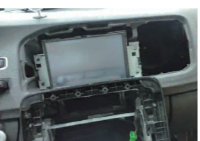
25. 将屏幕原来的插头重新插上，还原屏幕 Reconnect the original plug of the screen to the screen, and restore the screen
