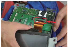
13. 将屏幕上的排线连接到CarPlay的PCB板上 Connect the flat cable of the screen to the PCB of CarPlay
