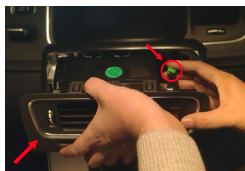
1. Remove the air-conditional panels and trim via plastic panel remover. (Note to disconnect the connector behind the panel)
