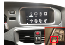
4. Long press EXIT button on the wheel to switch to carplay interface
