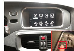
14. The installation is finished, put back all panels. Long press EXIT button on the wheel to switch to carplay interface
