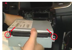
4. There are 2 screws on multimedia head unit, unscrew them and take out the box
