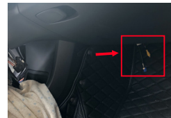
11. Put all harness through the ACC area to passenger glove box area. Recommend you put iSmart box here
