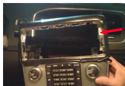
3. Remove the whole console control panel
