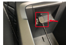
1. Insert the audio USB cable into car USB port.(if original car have AUX, omit this step)
