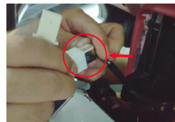
8. Connect CarPlay's LVDS cable with the original car's video
