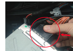
13. After the installation is complete, Insert the male side of the iSmart auto box 48PIN harness into head unit.
