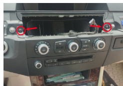
2. Unscrew the 2 screws on control panel.
