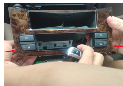
4. Take of the trim panel at bottom, note the connectors at 2 side
