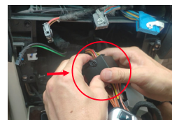
10. Connect the iSmart auto box 48PIN harness female side with original car 48PIN harness
