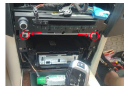
5. Unscrew the 2 screws on head unit.
