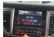
1. Press Source button to enter the original car audio source interface, select AUX
