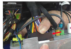
12. Connect the other end of the main CarPlay cable to the original car head unit car main line
