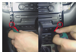
4. Unscrew the 2 screws on the head unit.
