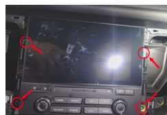
2. Unscrew the 4 screws on head unit.
