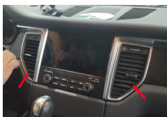
1. Remove the air-conditional panels and trim via plastic panel remover.
