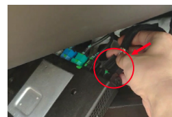
16. iSmart auto microphone was recommended to put in front of rear mirror area. (Hide the microphone cable) Connect with microphone cable
