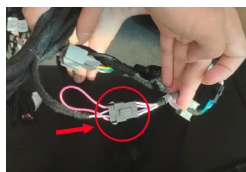
4. Unplug the Link cable on the main line of iSmart CarPlay and dock with the Link cable
