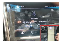
23. Keep phone WIFI ON, Open phone Bluetooth and searching (Find the Bluetooth name and pairing code of iSmart box). Insert pairing code
