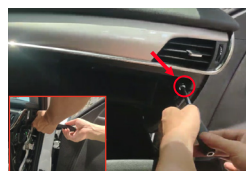
19. Connect the steering wheel control cable of iSmart CarPlay to the steering wheel, and connect it to original wheel control cable
