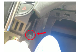
11. Unscrew the remaining screws of the glove box
