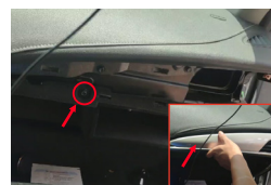
20. Connect the steering wheel control cable of iSmart CarPlay to the power cable (The wiring harness can be led to the position of the glove box from here)
